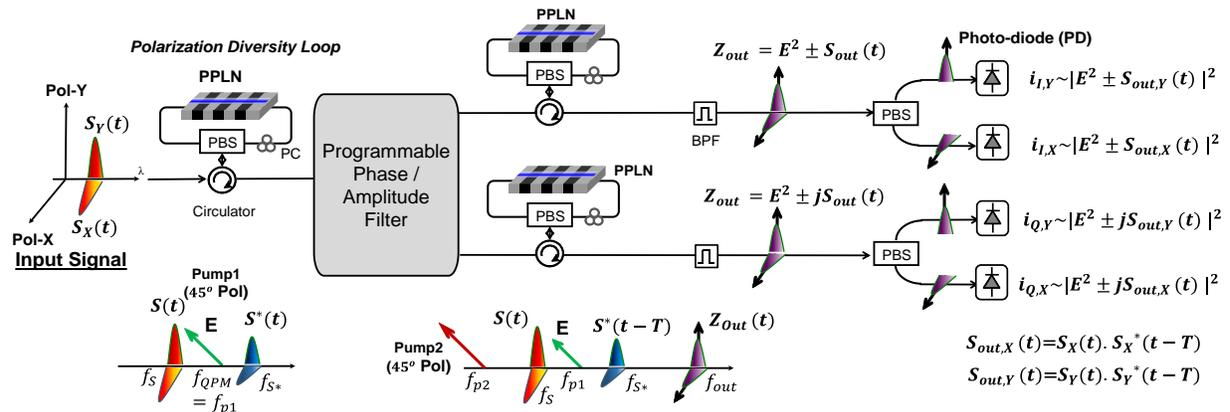
Fig. 1. Concept of the proposed homodyne detection scheme for polarization multiplexed signal.
