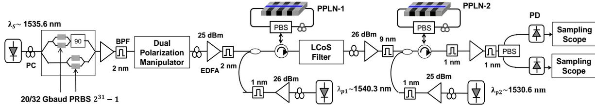
Fig. 2. Experimental setup. PC: Polarization Controller, BPF: Band Pass Filter, EDFA: Erbium Doped Fiber Amplifier
