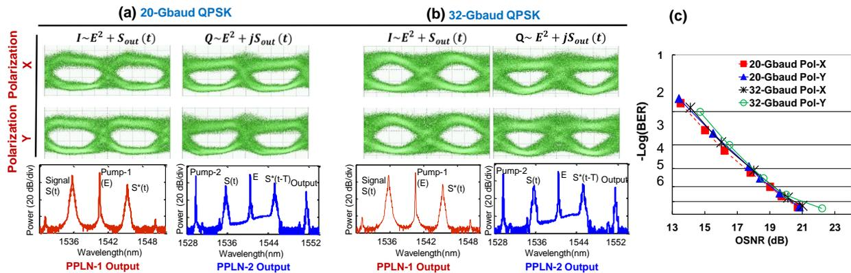
Fig. 3. Experimental results for proposed homodyne detection scheme of polarization multiplexed QPSK signals (a) Optical spectra of the PPLNs output and eye diagrams of I and Q for both polarizations of X and Y at 20 Gbaud. (b) Results at 32-Gbaud. (c) BER measurements.
