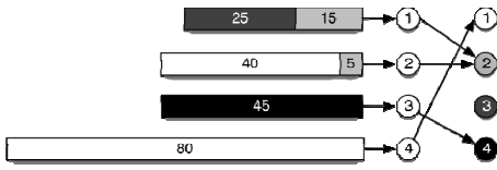
Figure 1: Head-of-the-line (HOL) blocking. Input port 1 and 2 are contending for output port 2. If the switch picks input port 2, then the second packet at input port 1 is HOL blocked.
