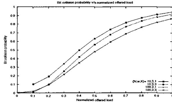
Fig. 2. Probability of a bit collision ( $P_m(w)$ ) against normalized offered load ( $m/N$ ) for different codeset design parameters ( $N, w, \kappa$ ) for Aloha-CDMA.
