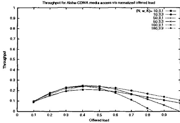
Fig. 3. Network throughput ( $T_{\text{aloha-cdma}}$ ) against offered load for different codeset design parameters ( $N, w, \kappa$ ) for Aloha-CDMA from analysis. The average packet length was 500 bytes and the chipping rate was 1Gb/s.
