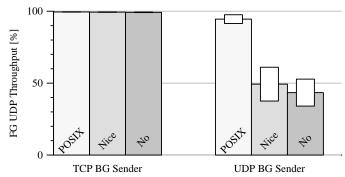
Figure II.1 Normalized mean throughput of a FG sender under unlimited load in the basic case ("No") and with two backgrounding mechanisms ("Nice" and "POSIX"), using TCP (left graph) and UDP (right graph) with 95% confidence intervals.
