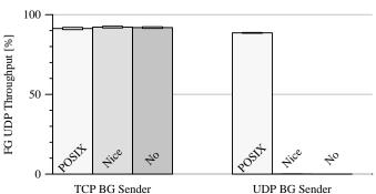
Figure II.2 Normalized mean throughput of a bursty FG sender in the basic case ("No") and with two backgrounding mechanisms ("Nice" and "POSIX"), using TCP (left graph) and UDP (right graph) with 95% confidence intervals.
