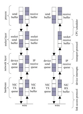
Figure III.3 Queueing at different layers for TCP (left) and UDP (right) processing.
