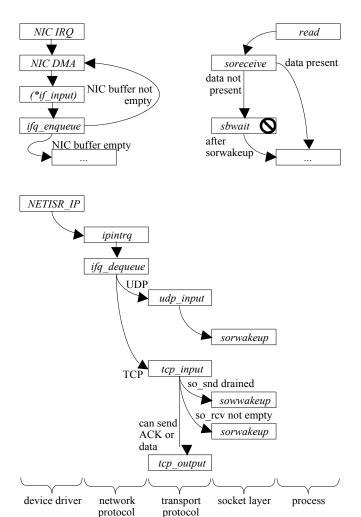
Figure III.2 Network stack inbound data processing.
