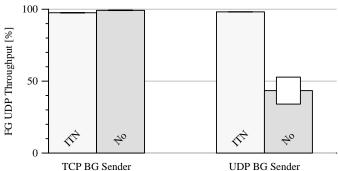
Figure V.1 Normalized mean throughput of a FG sender under unlimited load in the basic case (No) and with ITN backgrounding mechanism (ITN), using TCP (left graph) and UDP (right graph) with 95% confidence intervals.
