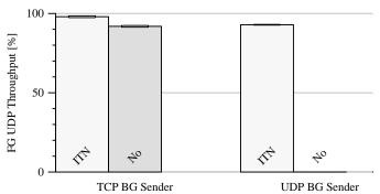
Figure V.2 Normalized mean throughput of a bursty FG sender in the basic case (No) and with the ITN backgrounding mechanism (ITN), using TCP (left graph) and UDP (right graph) with 95% confidence intervals.
