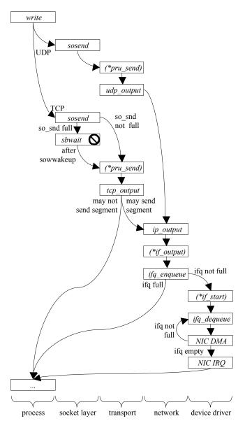
Figure III.1 Network stack outbound data processing.
