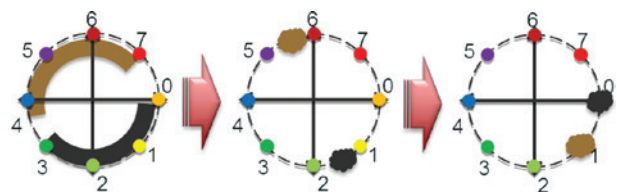
Figure 19: Half-phase add transformed into encoded carry out.
