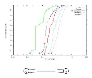
Figure 5: Web connection breakdown for ISDN with local requests with network diagram
