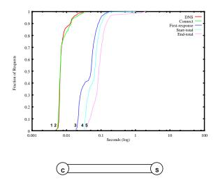
Figure 3: Web connection breakdown for LAN with local requests with network diagram
