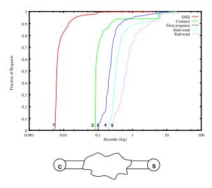
Figure 2: Web connection breakdown for LAN with remote requests and network diagram
