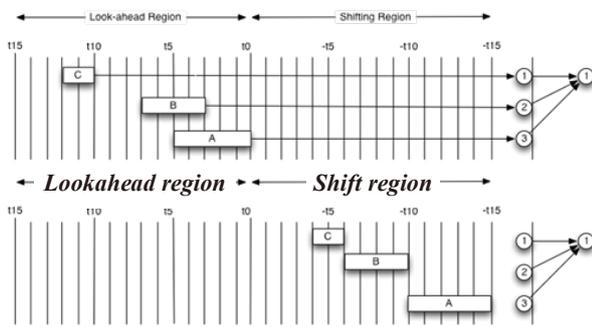
Fig. 3. Lookahead/shift effect on packet processing.
