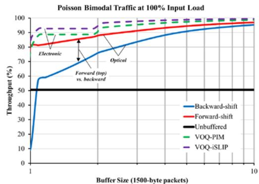
Fig. 4. Throughput comparison of 100% input load Poisson traffic.
