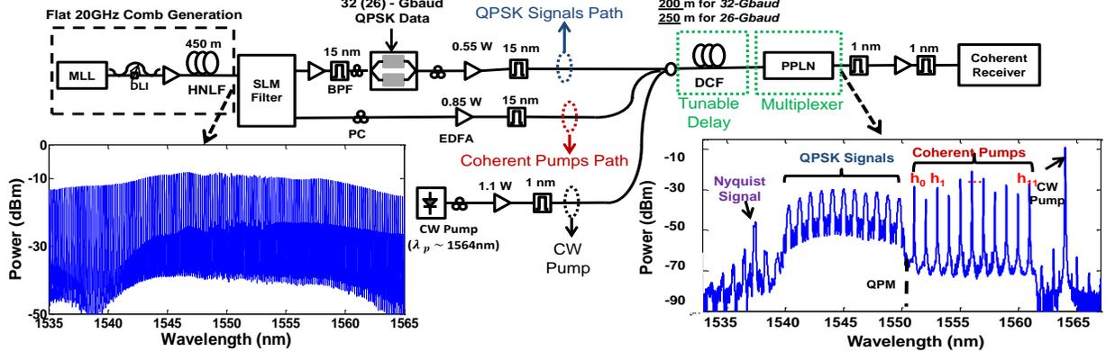
Fig. 2. Experimental setup. MLL: Mode Lock Laser, DLI: Delay Lin Interferometer, BPF: Band Pass Filter, PC: Polarization Controller,
