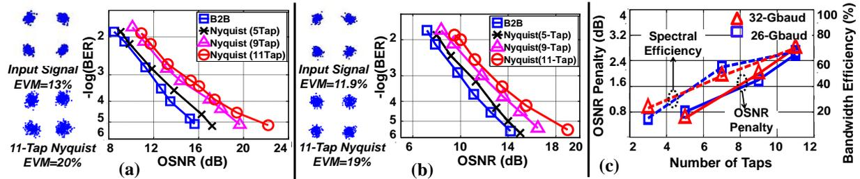
Fig. 4. *Experimental* results (a) EVM of input and output signal for 11-taps and BER measurements vs. OSNR of 32-Gbaud QPSK signal. (b) EVM of input and output signal for 11-taps and BER measurements vs. OSNR of 26-Gbaud QPSK signal (c) Measured OSNR penalty and bandwidth efficiency (percentage of bandwidth between two main ripples on obtained Nyquist signal over ideal Nyquist BW) vs. number of taps.
