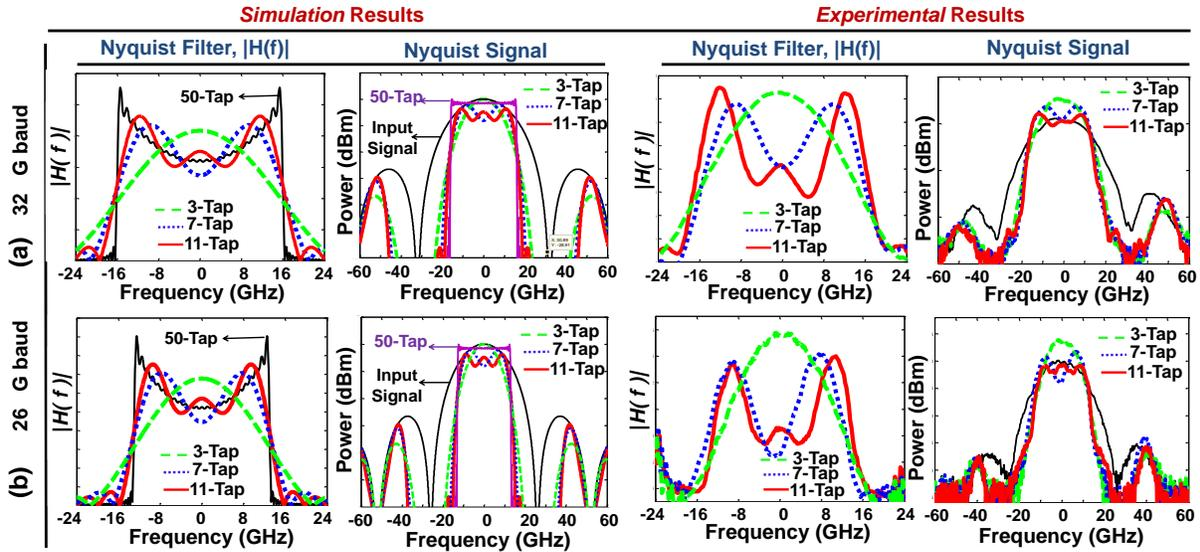
Fig. 3. Results of Nyquist filter shape, i.e.,  $|H(f)|$ , and Nyquist signal spectrum for different number of taps at. (a) 32-Gbaud. (b) 26-Gbaud.
