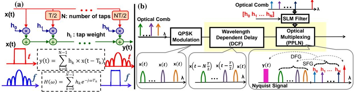
Fig. 1. (a) Concept of Nyquist FIR filter. (b) Concept of optical Nyquist generation using comb based OTDL (using optical comb as the taps of the FIR filter and utilizing DCF to delay the tapped signals and multiplexing the tapped delayed signals in a PPLN waveguide).
