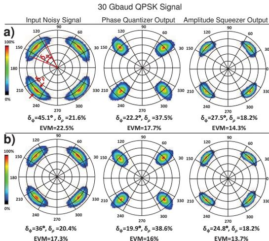
Fig. 4: Input/output constellation diagrams of phase noise mitigation for 30 Gbaud (a, b) QPSK signals impaired by different values of phase noise.
