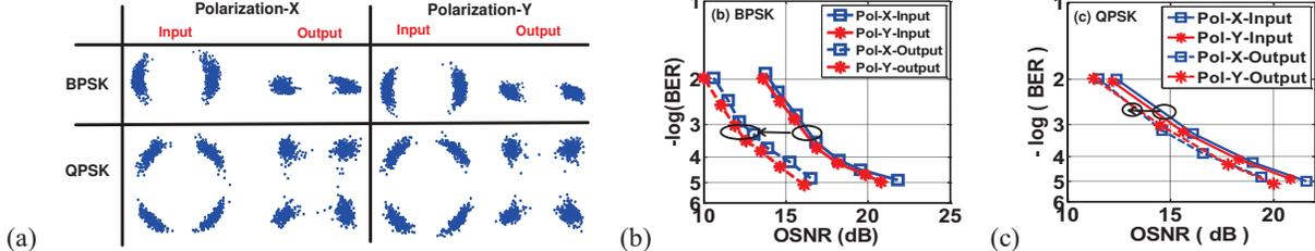
Fig. 3: Experimental results of DP-BPSK/QPSK regeneration. (a) Constellations of both polarizations. (b) BER measurements of DP-BPSK signals. (c) BER measurements of DP-QPSK signals.
