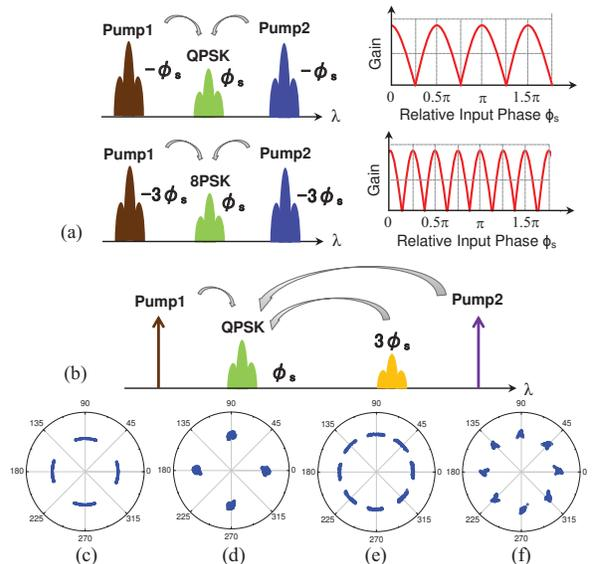
Fig. 1: (a) Degenerate scheme and transfer function for phase regeneration of QPSK/8PSK. (b) Non-degenerate scheme for phase regeneration of QPSK. (c) Non-regenerated QPSK (25Gbaud) with phase noise. (d) Phase-regenerated QPSK via degenerate scheme. (e) Non-regenerated 8PSK (25Gbaud). (f) Phase-regenerated 8PSK via degenerate scheme.
